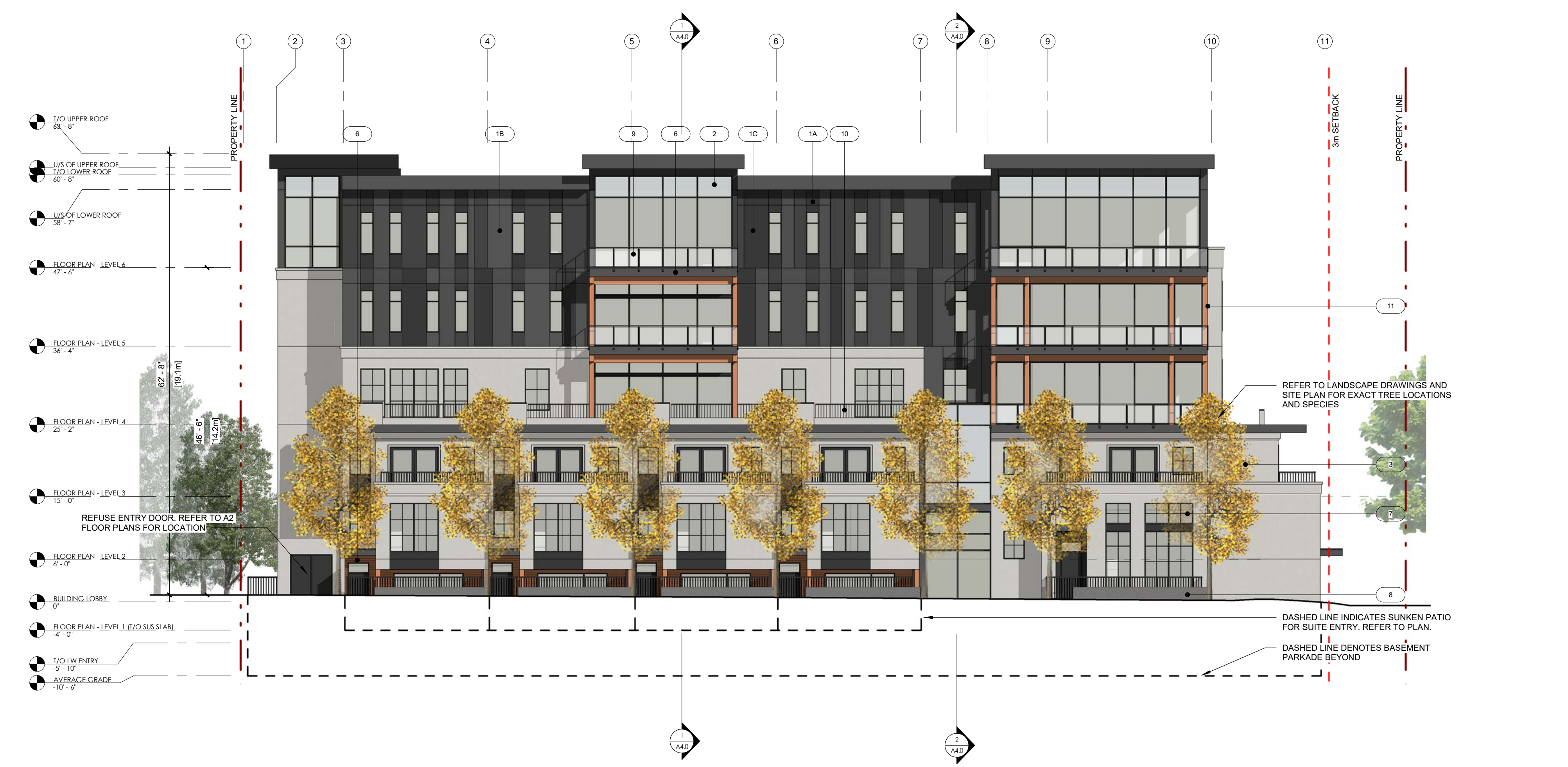
2 BUILDING ELEVATION - SOUTH 3/32" = 1'-0"
