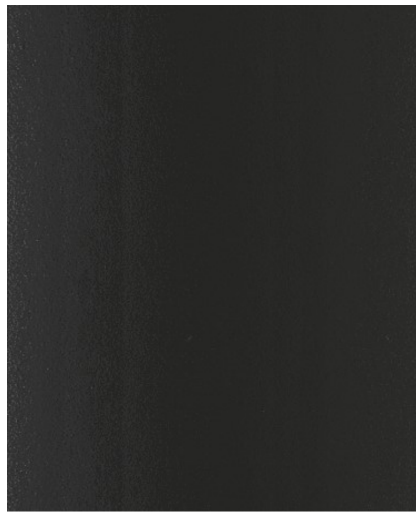
1A FIBER CEMENT PANEL COLOUR: IRON GREY MANUF/STYLE: SMOOTH SATIN FINISH, HARDI OR EQUAL
